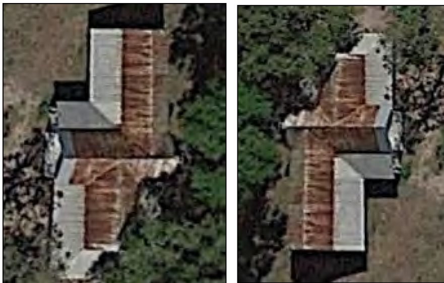
Figure 1. English Family House: 2018 aerials with south at bottom of left image and north at bottom of right image; T-shaped roofs of main block and linearly extended ell are topped by rusted roofs; porches and west gable end of main block are apparent from shiny appearance of re-clad roofs.
